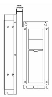
Fig. 2. "Side-by-side" installation
