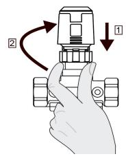
Tighten the connection union as shown below. Do not use additional tools as they may damage the actuator.
